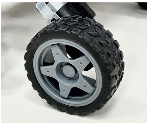
Figure 7 – Rover wheel tire tread with four lines of twenty-four tire blocks circumferentially organized.
