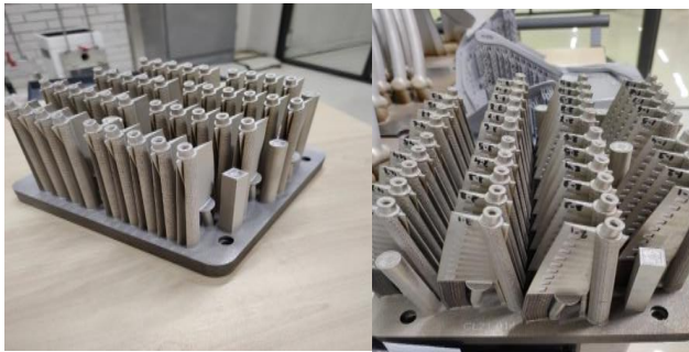
Fig. 1 rd blades obtained by selective laser sintering.
