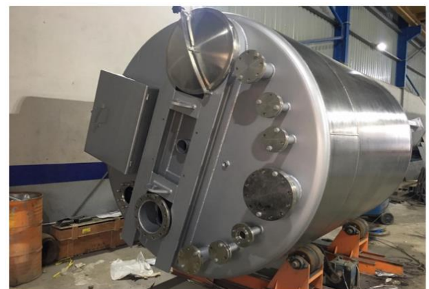
Figure 7: an assembly of the 30,000-liter acrylic storage reservoir
