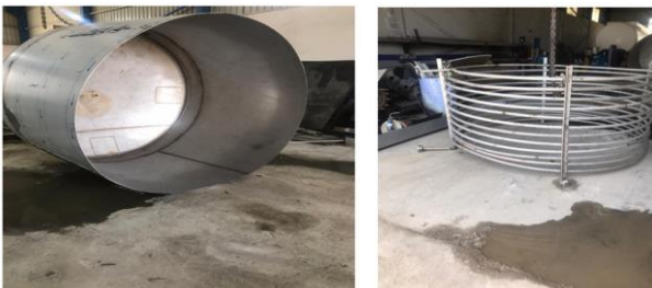
Figure 6: spiral heat exchanger in the lowest section of the reservoir before combination
