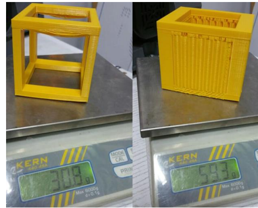
Figure 3: The mass of the printed cube without and with support structures
