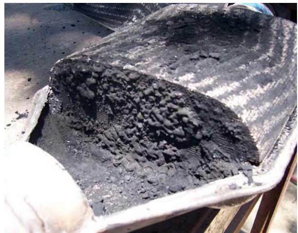
Fig 2: Blocked Diesel Particulate Filter[1]
