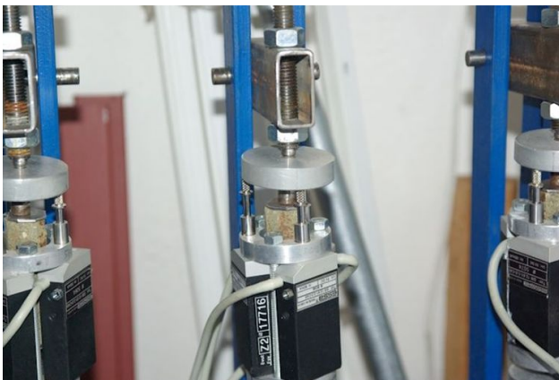
Figure 5: The instrumentation of the shrinkage test.
