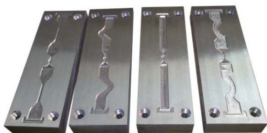
Fig. 4. Mold plates for individual test samples
