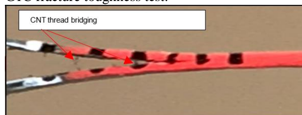
Fig 7. Double cantilever beam test for composites showing a 4-ply CNT thread stitched & CNT sheet patterned glass fabric composite test coupon. Multifunctional composite materials are being developed at the UC Nanoworld Laboratories for high rate manufacturing.
