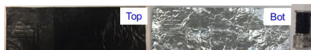
Figure 3. CNT-Al sheet top/bot and CNT yarn produced from the floating catalyst reactor sock.
