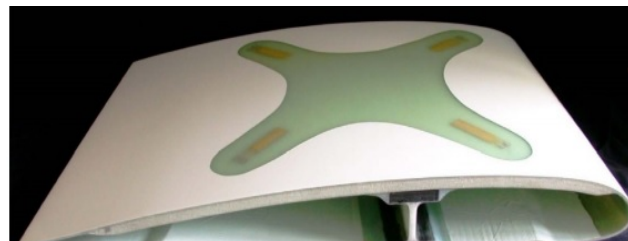
Fig. 8: Embedded PZT fiber transducer
