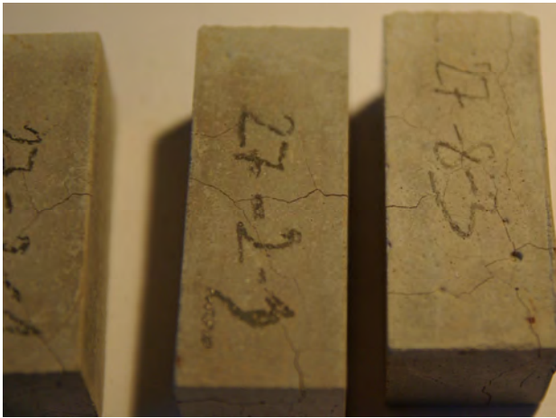
Fig.12 Specimens prepared for test of modulus of elasticity after temperature loading at 300 °C.
