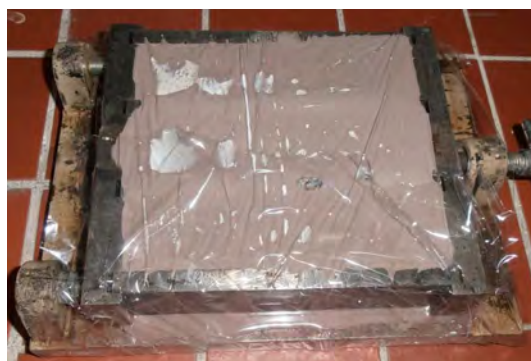
Fig.1 Concreting of cement paste into the steel forms. The foil covering the surface of the specimens against to leakage of moisture.
