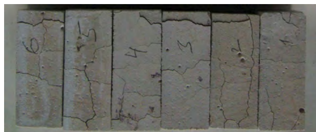
Fig.2 The specimen for material testing and after loading by temperature.
