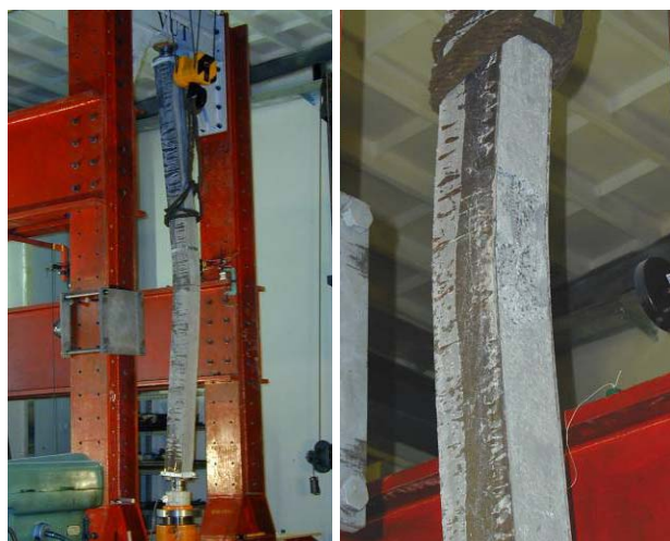
Fig. 1 Illustration of test arrangement and realization: HEA cross-section columns
