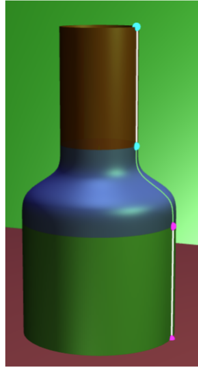
Figure 8: Two G^2 blends using a lathe from the curve in the Figure 6.
