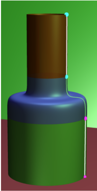
Figure 9: Two G^2 blends using a lathe from the curve in the Figure 7.
