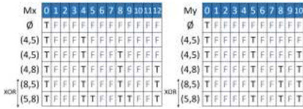
Figure 5: Example of Mx and My for the bin (12,10) and 4 objects: (4,5), (4,5), (4,8) and (5,8) with orientation free.
