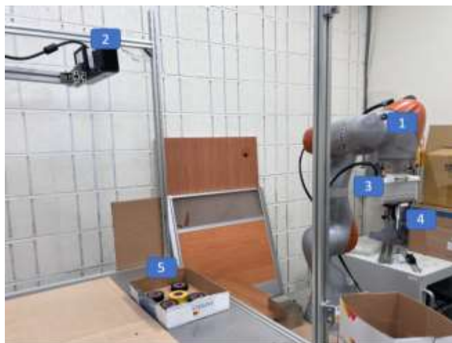
Fig. 2: Robotic painting system: (1) robotic arm, (2) RGB-D camera, (3) controller, (4) gripper, (5) grab object
