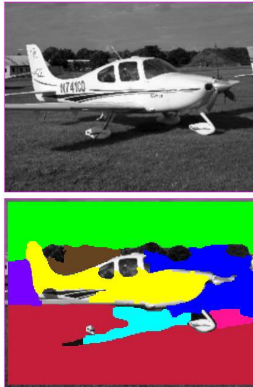
Fig. 3: The results of the texture segmentation on the example of processing a black-and-white image (upper part of the figure). The bottom half of the figure shows the largest texture segments highlighted in different colors
