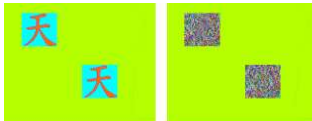
Fig. 9: An example of encryption of identical selected areas with different locations on the image of one video frame. Rule 105 was used with a shift by one step of evolution
