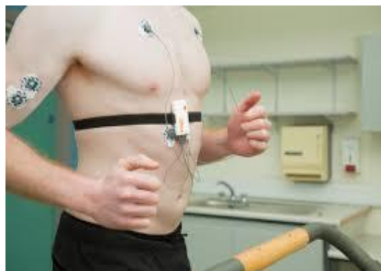
Fig.4 Sensors Directly Placed On Body for ECG Measurement
