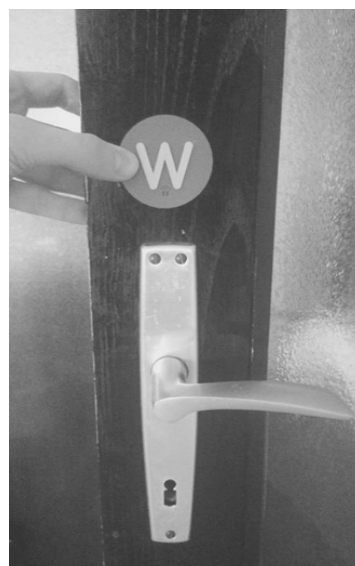
Fig. 2 Sensor node attached near the door lock
