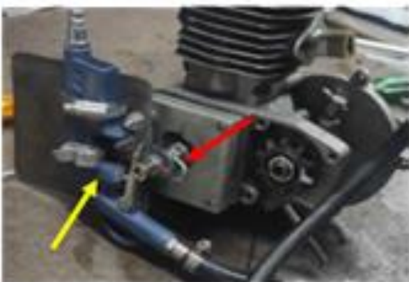
Fig. 10: The position of the air-gun, attached to the engine body (yellow arrow), and the almond that is screwed onto the crankshaft extension (red arrow) [3].
