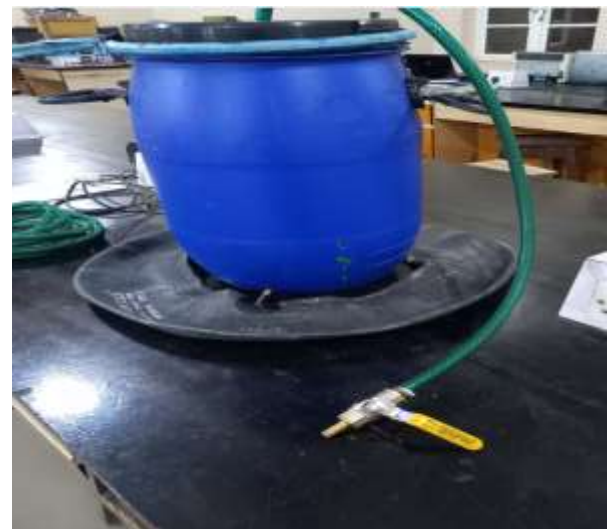
Figure 5. The Gas Tap Termination from the Fab Connected to the Cover of the Biogas Plastic
