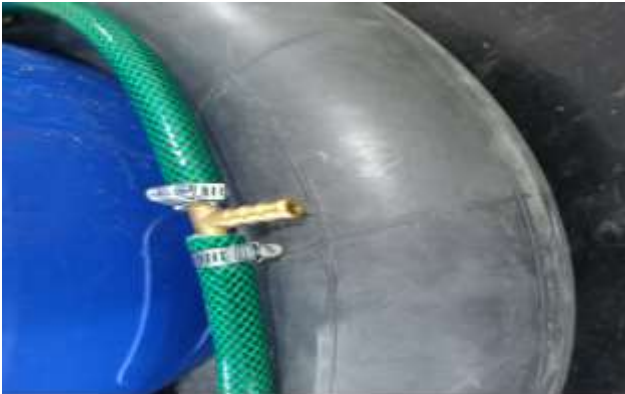
Figure 7. The Gas Tap was used in the Construction after the First Sets of Connection
