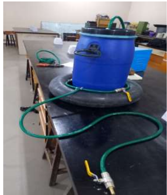
Figure 10. Barrel Drum Biogas Digester
