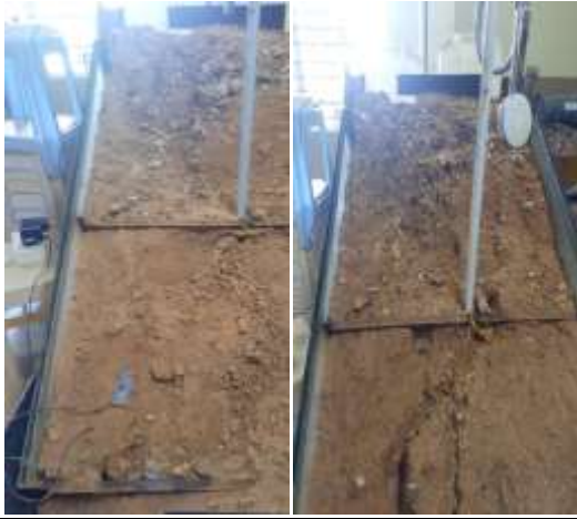
Figure 8: Initial and breakdown conditions when sensors are placed at one third distance
