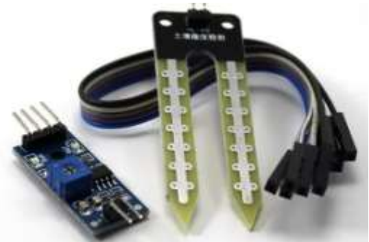
Figure 2: YL 38 soil moisture sensor
