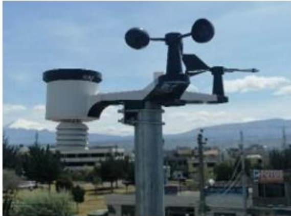
Fig. 3: Meteorological station, used to measure incident solar radiation and environmental variables Source: created by the authors
