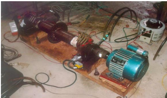
Fig 5: Testing setup of the experimental simulator when current supplied to the heating coils
