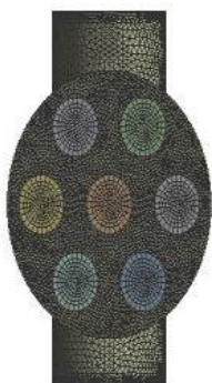
Figure 2: Grid generation over flow regime
