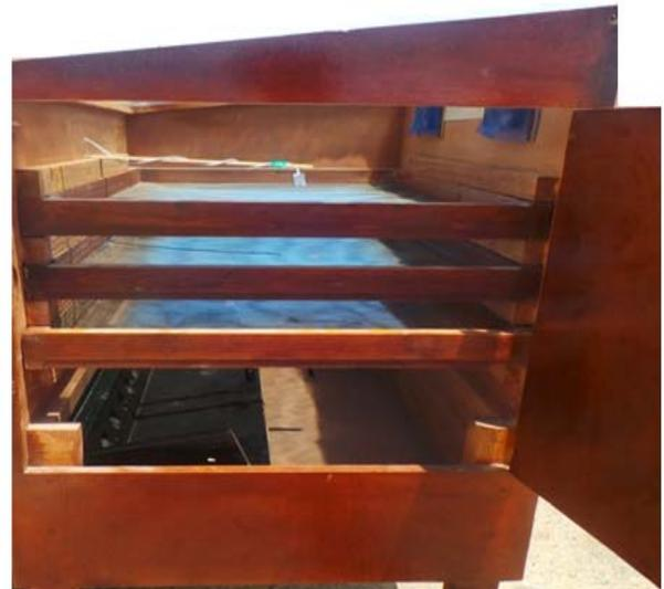
Fig. 2.2 Photo of the designed drying cabinet with its drying racks
