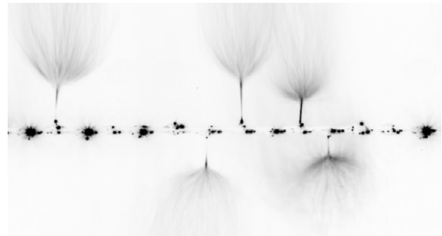
Fig. 3 Example of reflective method (inversed image) using collimated light - with good visibility flexural instability, but with significant spot reflections on drops on the spinning electrode (wire). Contour and shape of liquid are difficult to see.
