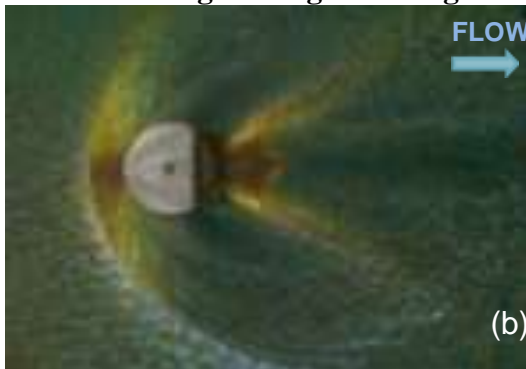
Fig. 8: Liquid Crystal Shear Stress Images showing Bow Shock and Wake distributions from 1.5mm and 3.0 mm wedge-shaped protuberances at Mach 4
