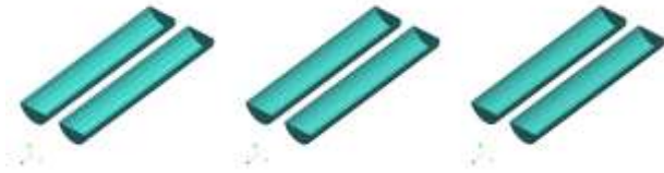
Fig. 4: Three mesh configurations used for the sensitivity analysis on the catamaran hull with L/a=5 and b/a=1.5 . Left to right: coarse, medium, and fine panel mesh
