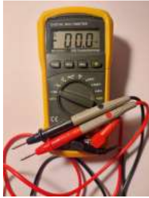
Fig. 16: Multimeter for voltage, current, and resistance measurement
