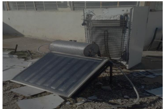
Figure 21. The pilot hybrid integrated Solar vapor compression fridge
