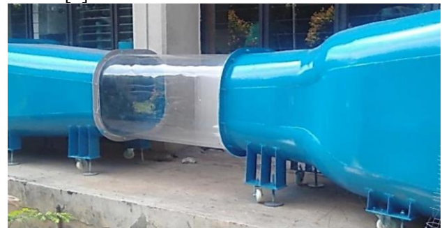
Fig. 2: The wind tunnel in Mechanical Engineering Laboratory
