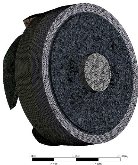
Figure 5: Mesh elements observed on the pump model
