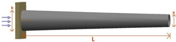
Fig. 1. Variable cross sectional Cantilever pipe containing flow fluid.
