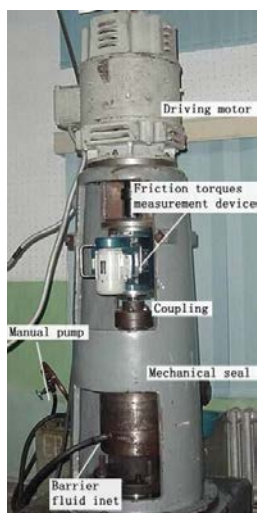
Fig. 12. The experimental device for measuring friction torques
