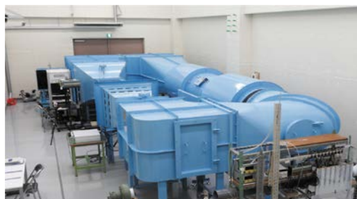
Fig. 1 Overall view of wind tunnel
