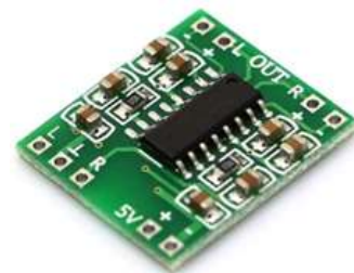
Fig.3. Block diagram and appearance of the PAM8403 (HW-104) audio amplifier chip
