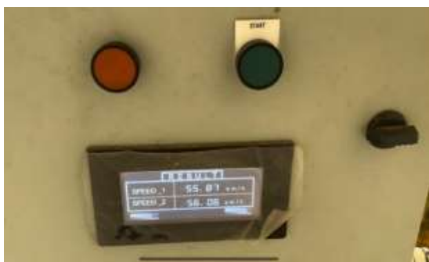
Fig. 6: Vehicle speed displayed on the crash test control panel
