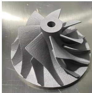
Fig. 4. Product of turbine blades after 3D printing
