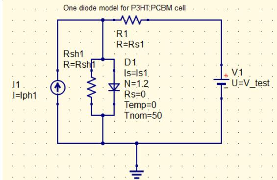
Fig. 3. Equivalent circuit model used under QUCs simulator.
