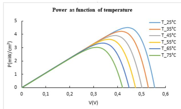
Fig. 5. Simulation of the power generation of the cell as function of temperature.
