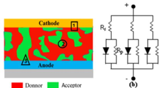
Fig. 8. (a) Schematic representation of the three junctions in organic solar cells: (1) the donnor/cathode junction, (2) the internally distributed donnor/acceptor junction and (3) the acceptor/anode junction, (b) equivalent circuit of the three junction model.
