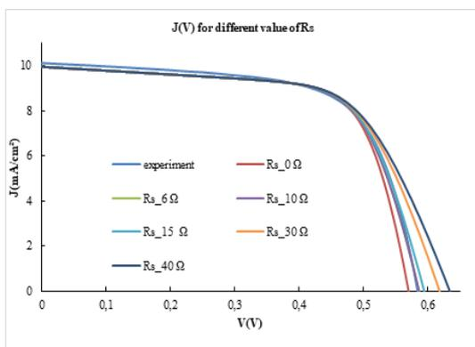
Fig. 7. Simulation of J(V) characteristics as function of the series resistance
