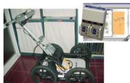
Figure 7. The GPR system that used for this survey
