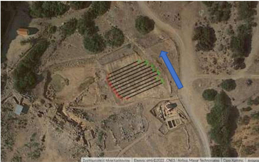
Figure 3. Profiles of measurements made in subarea A. The start point is shown in green dot and the end point of each section is shown in red dot. The arrow indicates the scanning direction (from bottom to top – point X=0m and Y=0m corresponds to the lower right green dot)
