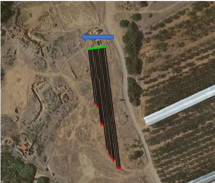
Figure 4. Profiles of measurements made in subarea B. The start point is shown in green dot and the end point of each section is shown in red dot. The arrow indicates the scanning direction (from right to left - point X=0m and Y=0m corresponds to the upper right green dot)
