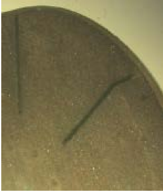
Fig.7 Channels and holes in the abrasive bodies.
