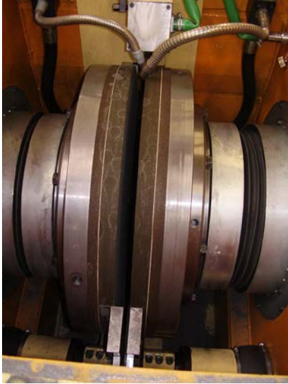
Fig.4 Penetration of the cutting fluid from the top of the grinding bodies.
