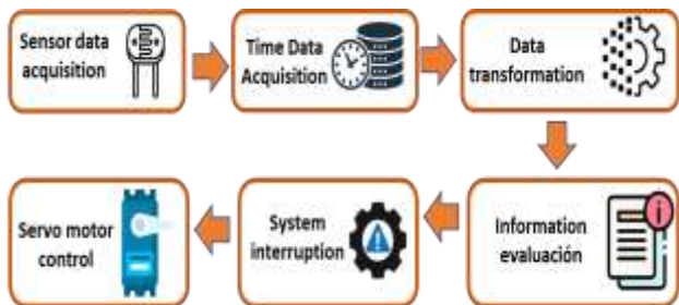
Fig. 5: Block diagram of the control algorithm for solar tracking
