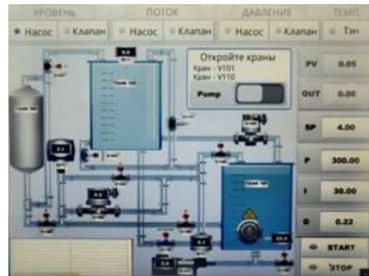
Fig. 2: SCADA Human Machine Interface
