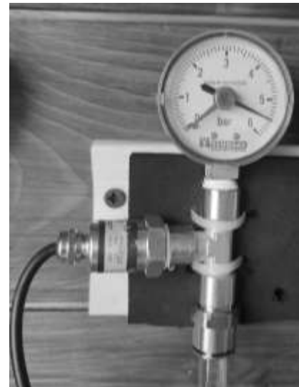
Fig. 6: Setup for the pressure sensor calibration.
