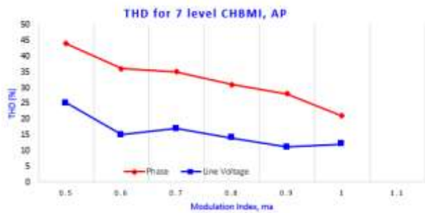
Fig. 9: THD of output voltage performance for CHBMD using PD strategy for different m_a values
