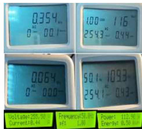
Fig. 5: Power analyzer and LCD readings for the 100-watt Lamp load
