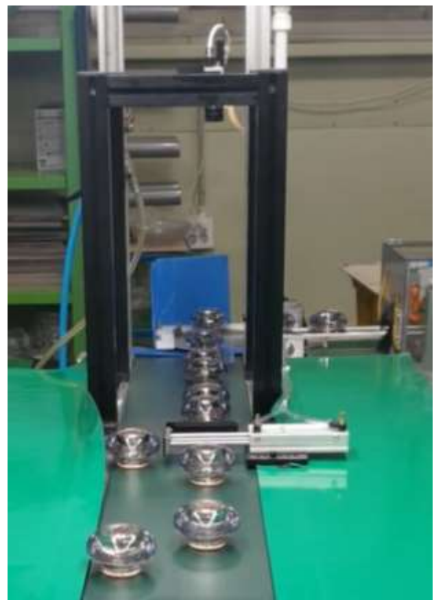
Fig. 6: Discharge of the identified defective product
