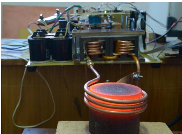
Fig. 5: The process of induction surface heating of metal with a diameter of 120 mm at a frequency of 20 kHz.
