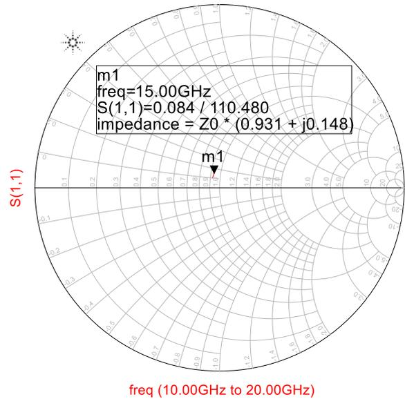
Fig.2. Input impedance for common-gate structure
