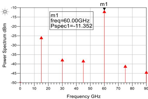
Fig.3. Power levels of different harmonics of unmached frequency multiplier by 4
