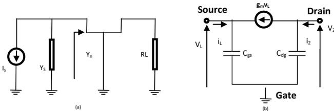
Fig.1. (a) Common-gate - (b) Small signal equivalent circuit
