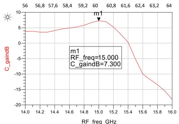
Fig.6. Power evolution of conversion gain a function of frequency of mached frequency multiplier
