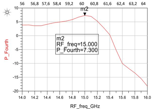
Fig.5. Power evolution of the fourth harmonic as a function of the input/output frequency of mached frequency multiplier
