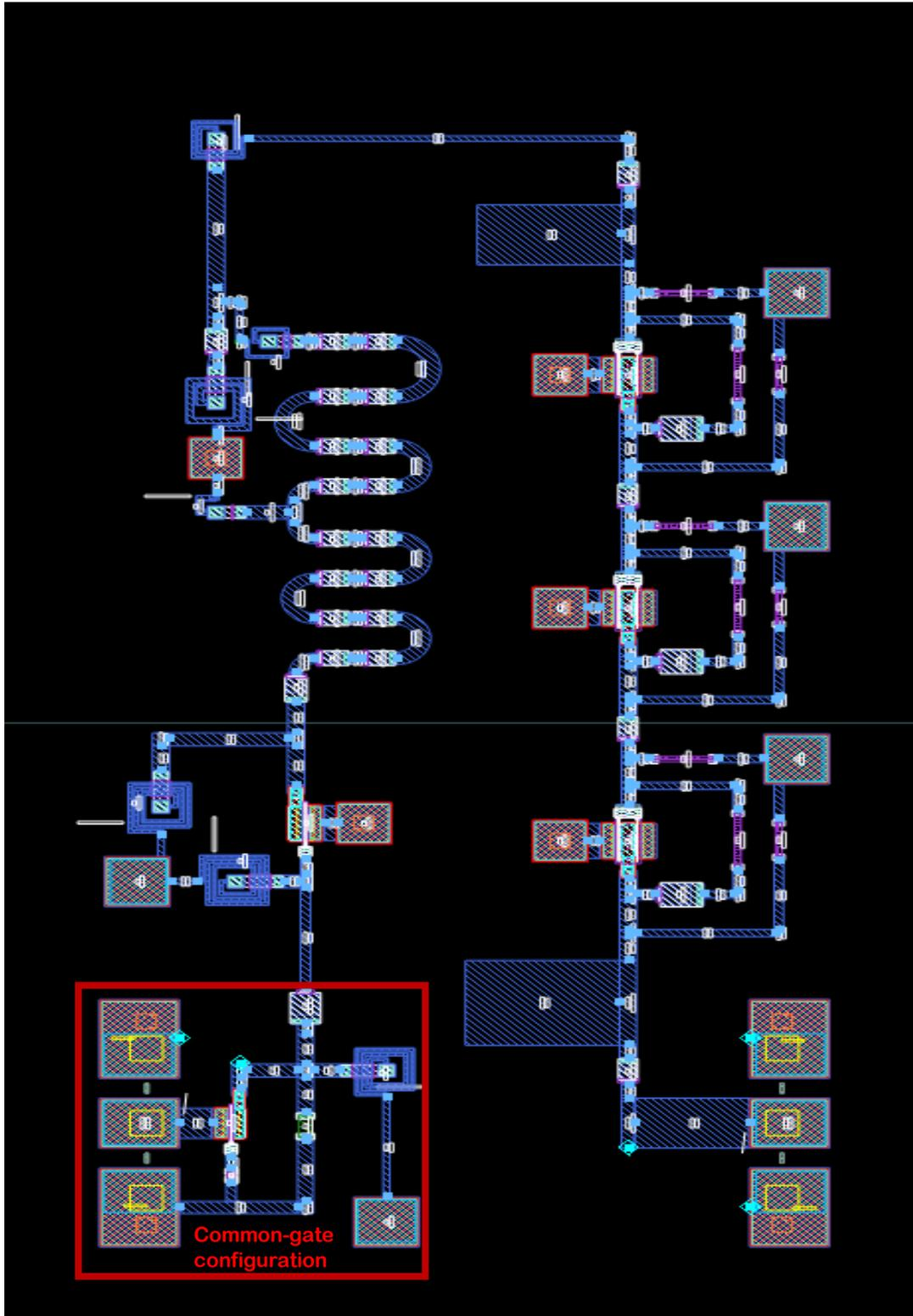
Fig.7. Layout of frequency multiplier by 4 with common-gate configuration
