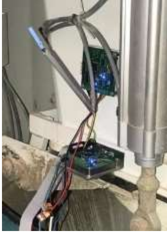
Fig. 2. Control system connected to active weighing system
