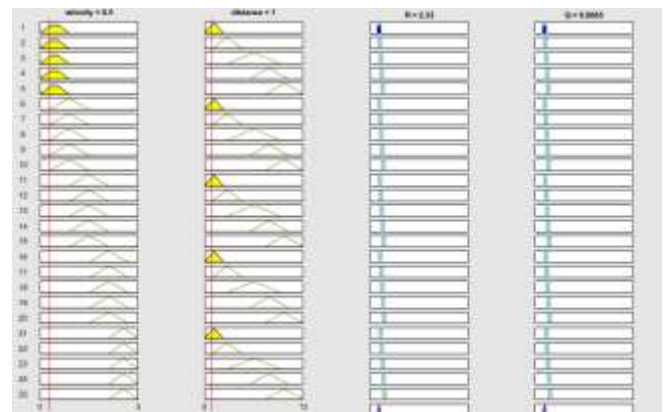
Fig. 16. Sugeno Fuzzy Logic Inference Example for Input Speed=0.5 and Position=1, Q=0.1 R=2
